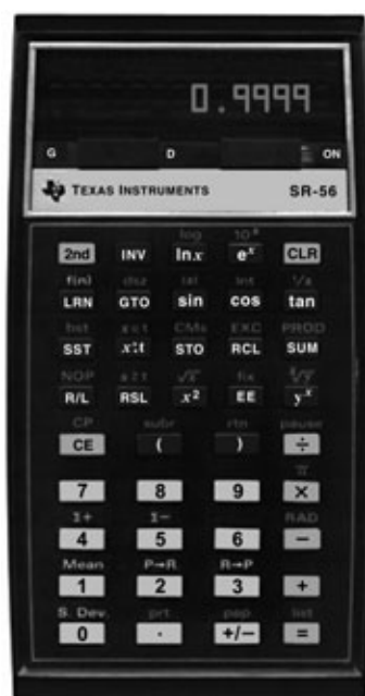
Fig. 1.8. Programmable pocket calculators Model SR-56 of the Texas Instruments Corporation and Model HP-67 of the Hewlett-Packard Corporation, both first manufactured in 1976. Seven-segment numeric characters composed of GaAsP LEDs were used in the display. The SR-56 came with a “huge” program memory of 100 steps. The HP-67 came with a magnetic card reader and had several freely programmable keys.
