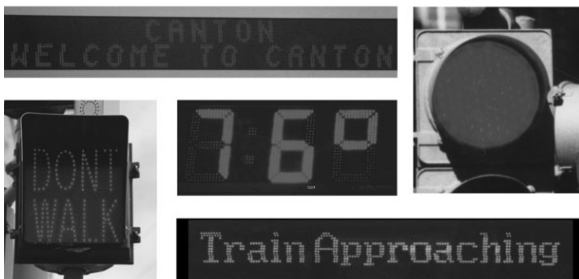
Fig. 1.12. Examples of red and amber AlGaInP/GaAs LEDs used in signage applications.
