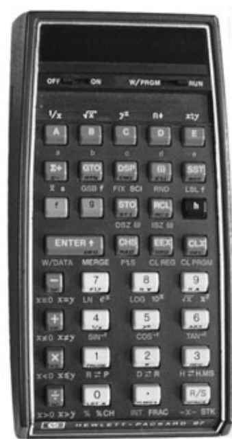
Fig. 1.8. Programmable pocket calculators Model SR-56 of the Texas Instruments Corporation and Model HP-67 of the Hewlett-Packard Corporation, both first manufactured in 1976. Seven-segment numeric characters composed of GaAsP LEDs were used in the display. The SR-56 came with a “huge” program memory of 100 steps. The HP-67 came with a magnetic card reader and had several freely programmable keys.
